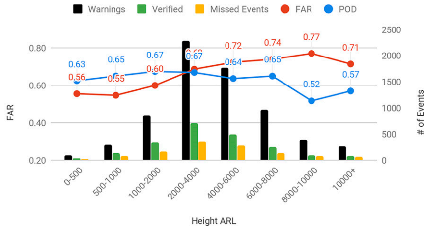
FIG. 8. FAR (red) and POD (blue) per height ARL range bin. Bar chart also shows warnings (black), verified warnings (green), and missed events (yellow).
